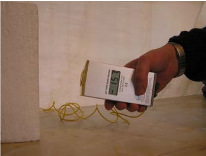
Using a fieldmeter to detect and measure the surface voltage of charged polystyrene foam
